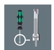
A screwdriver with a hollow shaft is needed whenever there are screwdriving jobs involving threaded rods i.e. the threaded rod through the nut can slip into the hollow shaft of the screwdriver.
