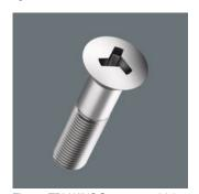
TRI-WING® screwdriving The system is mainly found in aviation and household technology (here e.g. on live components). The asymmetric arrangement of the three profile flanks prevents the use of anything other than the original tools. The high-precision Wera profile design ensures a secure fit of the tool in the head of the screw. The blades are manufactured out of bit material. The Wera know-how with regard to the hardening technology ensures a long service life of the tool.
