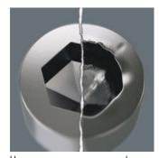
Hexagon screws can endure a problem because the contact surfaces delivering the power from conventional tool, transferred to the screw via very small surface areas. The consequence: the screw can become damaged (rounding out). Hex-Plus tools have a greater contact surface that prevents this from happening! At the same time, as much as 20 % more torque can be applied. Good to know: Hex-Plus tools fit into every standard hexagon socket screw!
