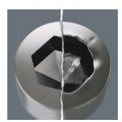
Hexagon screws can endure a problem because the contact surfaces delivering the power from the conventional tool. transferred to the screw via very small surface areas. The consequence: the screw become damaged (rounding out). Hex-Plus tools have a greater contact surface that prevents this from happening! At the same time, as much as 20 % more torque can be applied. Good to know: Hex-Plus tools fit into every standard hexagon socket screw!
