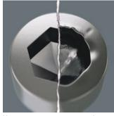
Hexagon screws can endure a problem because the contact surfaces delivering the power from conventional tool, is transferred to the screw via very small surface areas. The consequence: the screw can become damaged (rounding out). Hex-Plus tools have a greater contact surface that prevents this from happening! At the same time, as much as 20 % more torque can be applied. Good to know: Hex-Plus tools fit into every standard hexagon socket screw!
