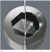
Hexagon screws can endure a problem because the contact surfaces delivering the power from conventional tool, is transferred to the screw via very small surface areas. The consequence: the screw can become damaged (rounding out). Hex-Plus tools have a greater contact surface that prevents this from happening! At the same time, as much as 20 % more torque can be applied. Good to know: Hex-Plus tools fit into every standard hexagon socket screw!
