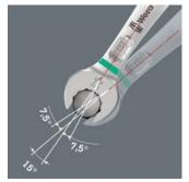
Thanks to the 7.5° offset open end, the double hexagon geometry and an improved application method (placement - screwdriving - rotation - re-placement screwdriving - rotation etc), even screwdriving situations that have a return angle of less than 30° can be solved.
