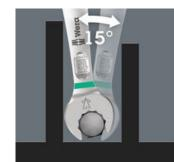
The Joker 6005 double open end wrench with its special open end design - a 7.5° offset open end and double hexagon geometry -doubles the placement points at a repeated 180° rotation of the wrench around the longitudinal axis. Bolts and screw heads can be engaged every 15°. The Joker 6005 will automatically find the respective placement point after every turn.
