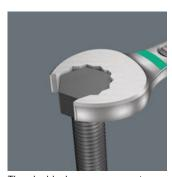
The double hexagon geometry on the open end and ring sides secures the positive connection with the screw head or bolt and reduces the risk of slipping.
