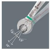
Thanks to the open end side offset by 7.5°, double hexagon geometry and an adjusted application method (placement - screwdriving - turning - replacement screwdriving - turning, etc), even screwdriving challenges allowing a return angle of less than 30° can be solved.
