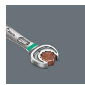
The Joker's clever double-hex geometry delivers a very positive connection with nuts or bolts - it's a perfect fit. And the exchangeable, hardened metal gripping plate in the Joker's open end literally bites itself into the bolt, with its extremely hard tips. Both features combine to prevent slipping, even at higher torque. Fine tooth mechanism
