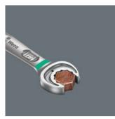
The Joker's clever double-hex geometry delivers a very positive connection with nuts or bolts - it's a perfect fit. And the exchangeable, hardened metal gripping plate in the Joker's open end literally bites itself into the bolt, with its extremely hard tips. Both features combine to prevent slipping, even at higher torque. Fine tooth mechanism
