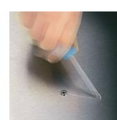
It happens time and time again that the tip slips out of the screw when screwdriving, head sometimes damaging valuable surfaces or even causing injury. The tips of the Wera Lasertip screwdrivers are microscopically roughened by means of a laser. This rough surface literally "bites" itself firmly into the screw head. Slipping out becomes a thing of
