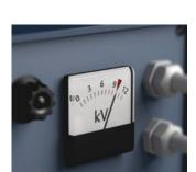
The individual testing at 10,000 volts, in accordance with IEC 60900, ensures safe working with loads up to 1,000 volts.
