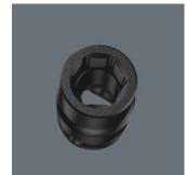
The hexagon profile allows the transmission of high forces and puts less strain on the edges of bolts or screw heads than a double hexagon profile. Fine-toothed ratchets also make the use of a double hexagon profile superfluous, even in confined spaces, thanks to their small return angle.
