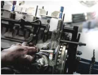
Nutsetter for hexagon head screws
