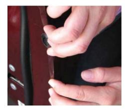
**8.** After starting to secure the edge, continue to fold the film around to the back of the door edge over the entire length of the door.
