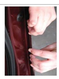
9. Remove all air bubbles by smoothing with moderate finger pressure.
