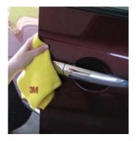
**3.** Always check part position, shape and size before applying. The Door Edge film is rounded on the ends; if desired it can be cut straight.
