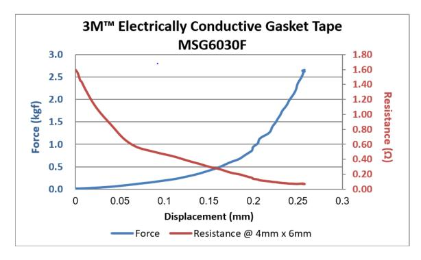
Force-Displacement-Resistance (FDR) Measurement Curves
