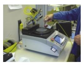
7. Apply de-ionized or distilled water. Using about 3 pumps of the spray bottle or enough to cover the surface of the film.
