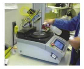
4. Wipe the surface of the 3M<sup>TM</sup> Lapping Film with a clean tissue. The goal here is to remove the air bubbles, smooth out the film and clean the surface of the film. The film should be wiped until almost completely dry and laying flat.
