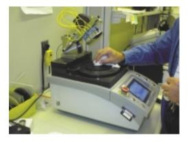
**Note:** The rubber back-up pad should be in good condition, with no scratches, gouges or foreign material on the surface. Additional cleaning or replacement may be necessary.
