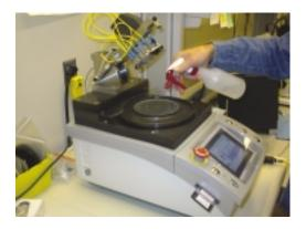
8. Lower the fixture, gently, taking care to not gouge the film. It is best to hold the fixture against the arm while moving the arm to the horizontal position. Once the arm is locked in place, the connector ends can be manually brought in contact with the lapping film, by lowering the fixture.
