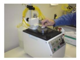
5. The film should be well adhered to the back-up pad, laying smooth and clean.
