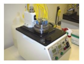
After the cycle, carefully lift fixture, to minimize scoring of the film, then move the fixture out of the way. The film can be wiped dry, and placed in a clean area for the next use.
