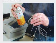
Applying contact cleaner to fixture with connectors.
