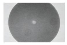
Ceramic Connector Cleaned with Novec Contact Cleaner
