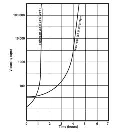
Brookfield Viscosity vs. Time 77°C and 93°C
