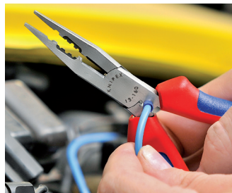
Crimping 20-14 AWG (0.5 to 2.5 mm 2 )
