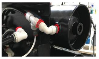
4. Connect Provided Tubing: PRODUCT (purified water - blue tubing) and CONCENTRATE (drain - black tubing) to their ports; re-direct the open ends of both the PRODUCT (purified water – blue tubing) and CONCENTRATE (waste water – black tubing) to drain. Install the red clips included in systems parts bag. Fully close the blend valve by turning it clockwise.
