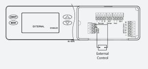
The Model A710V3 can be controlled with the Model A77 Control (included) or any external control that can provide a dry contact closure. When the Model A77 is used, the User Interface on the dehumidifier **MUST BE** set to "Remote". For all other external controls, the User Interface **MUST BE** set to "External". Refer to the quick start guide or installation manual for instructions on accessing the installer set-up menu.
