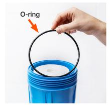
Clean o'ring and o'ring seat, then re-grease with food grade silicon grease.
