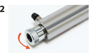
Make sure housing collar is firmly tightened. Do not over tighten as this will cause glass inner sleeve to break.
