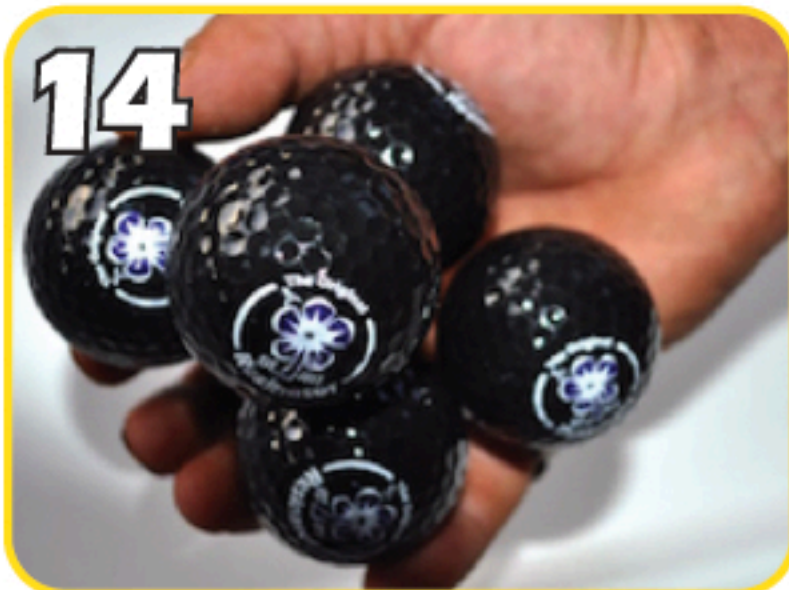
Apply agitation (balls, dry-ice, or ice) depending on extraction method, to drum interior with material. (See extraction guide) *Remove between loads for reuse. *Not necessary in wet operation.
