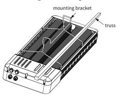
STEP 5: The truss size should be less than φ40mm /40\*40mm.
