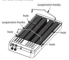
STEP 3: Hang the mounting bracket at the positions of suspension hooks
