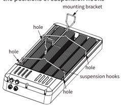
STEP 4: Hang the Mounting bracket on the truss
