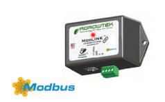
GrowNET<sup>™</sup> devices are easy to implement on PLC systems with MODBUS RTU and a LX2 ModLINK interface. Multiple GrowNET<sup>™</sup> devices can be connected to an interface with HX8 GrowNET<sup>™</sup> hubs.
