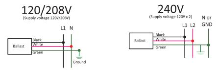
Each ballast **MUST** be wired to the main's neutral line back to the circuit. **DO NOT** "daisy-chain" a neutral line with any other ballast.
