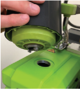
FIGURE 7: Demister removed, showing oil opening
