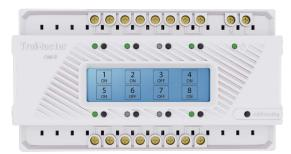
The OM-8 allows up to 12 Amp current through each contact. It should be mounted inside an electric control cabinet, and connected to a power supply between 100-240 VAC.
