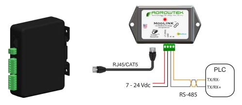
3.3/5Vdc Serial Bus Compatible. Include required bus terminating resistors per EIA standard.
