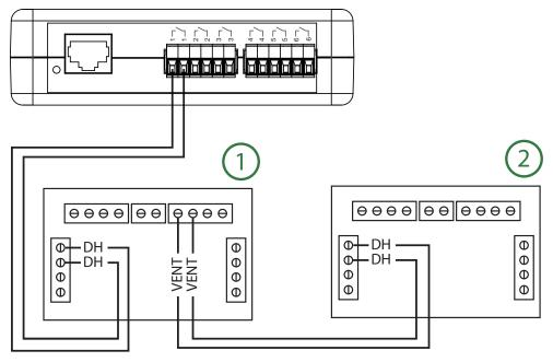
Connect the "DH" contacts of unit #2 to the "VENT" contacts of unit #1. Refer to Anden operation manual for additional setup instructions.
