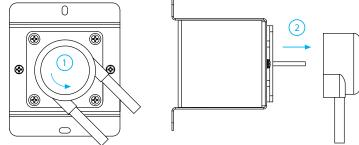
Re-install the head onto the shaft (align to the flat on the shaft) and twist-lock the head into position.
