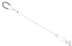
4 Steel Hanging Cables with attached cylindrical locks for hanging
