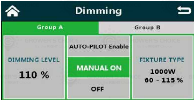
Displays power level in percent and watts. Touch this tab to access the "Dimming Menu"
