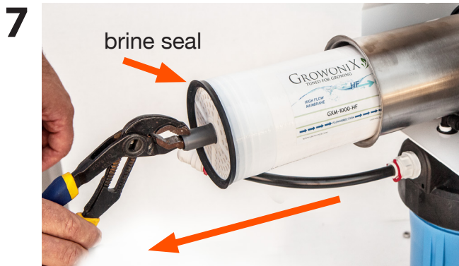
Pull the old membrane element out towards the input side of the membrane housing.
