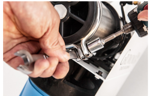
Tighten the stainless clamp retaining bolts evenly.
