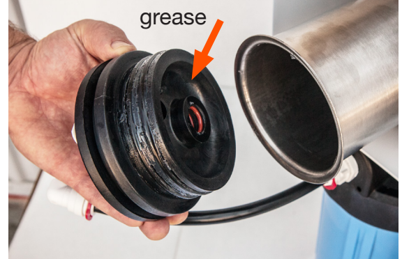
Grease the brine seal and end-cap center hole with food grade silicone grease.
