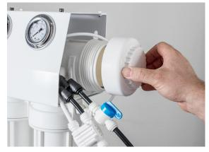
Unscrew membrane housing end cap. Caps can be difficult to remove. Be sure to have a firm grip on opposite side of housing.
