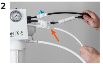
Connect 3/8" white RO tubing to the auto shut-off valve, making sure RO tubing seats all the way in quick-connect fitting.
