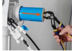
Pull out membrane using needle nose pliers or other similar tool.
