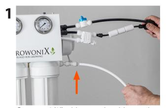
Connect 3/8" white supply tubing to the inlet fitting, making sure inlet seats all the way in quick-connect fitting.
