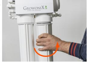
Tighten filter housings by hand, then finish with a 1/8 turn via the supplied filter wrench. Do not over tighten.
