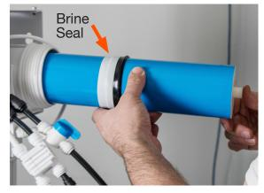
Lubricate the brinie seal and orings. Insert new membrane into housing, making sure the membrane-end with the brine seal goes in last. Make sure the membrane is completely seated in the housing.
