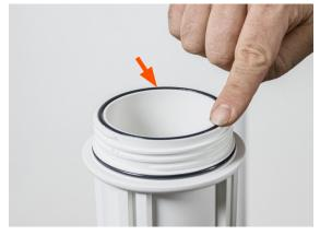
When replacing filter housings, make sure housing O-rings are seated properly. O-rings function best when lubricated with food grade silicone lubricant.
