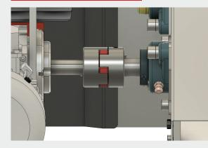
The Lovejoy coupling should be installed so both metal jaws are touching the raised dots on the plastic spider. If further adjustment is needed, the metal jaws can be adjusted by loosing the set screw on the metal jaws and moving them in or out on the shaft to achieve the correct fit.
