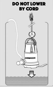
**PLACE BOTH TIPS OF** STABILIZING FOOT AGAINST SIDEWALL OF TANK
