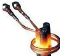
Small steel rod heat treat
