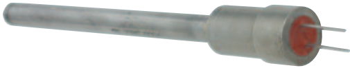
Cartridge heater for continuous air heating application with Incoloy® sheath, custom machined fitting and silicone rubber moisture barrier.
