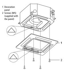
After installing the decoration panel, ensure that there is no space between the unit body and decoration panel. Otherwise air may leak through the gap and cause dewdrop (See figure below).
