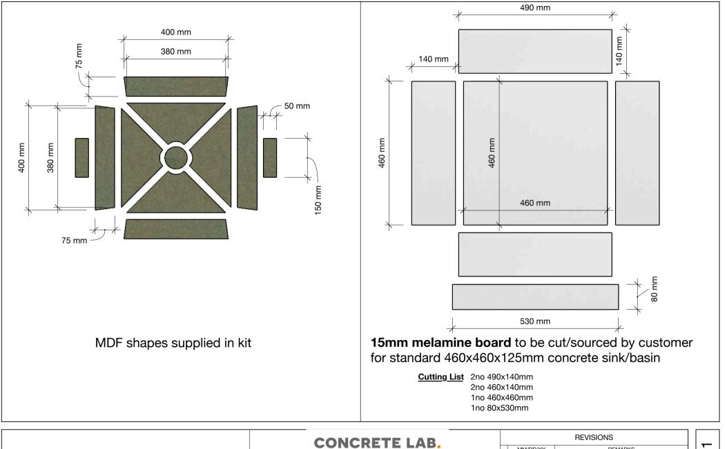
Medium Sink Insert Mould & Outer Parts
