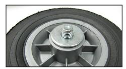
Wheel with 5/8" bolt and washer in place.
