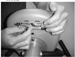
Note: Ensure batteries are properly installed in the correct direction as indicated by battery and polarity symbols in console battery case.
