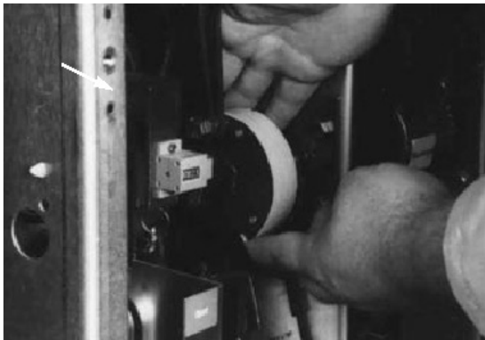
Figure 32. Attaching tape around to the back of the cam.
