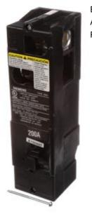
Siemens Low Voltage Residential Circuit Breakers Main Breakers - Type QS Breakers are Circuit Protection Load Center Mains, Feeders, and Miniature Circuit Breakers. Type: QSH Application: Electrical Distribution Standard: UL 489 Voltage Rating: 120/240V Amperage Rating: 200A Trip Range: Thermal Magnetic Interrupt Rating: 22 AIC Number Of Poles: 2P
