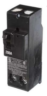
Siemens Low Voltage Residential Circuit Breakers Main Breakers -Branch Main Breakers Non-reversible are Circuit Protection Load Center Mains, Feeders, and Miniature Circuit Breakers. Type: QN Application: Electrical Distribution Standard: UL 489 Voltage Rating: 120/240V Amperage Rating: 200A Trip Range: Thermal Magnetic Interrupt Rating: 10 AIC Number Of Poles: 2P
